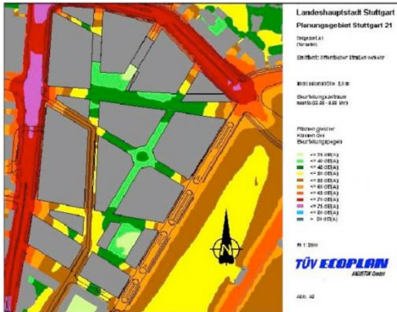
Noise emission plan Road traffic, current state Plan area A1 during the night
