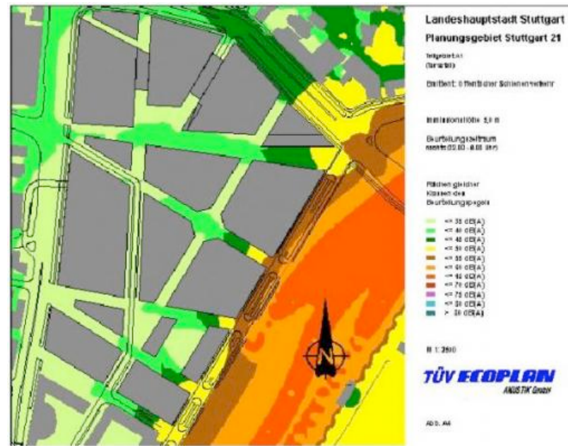
Noise emission plan Railway traffic, current state Plan area A1 during the night
